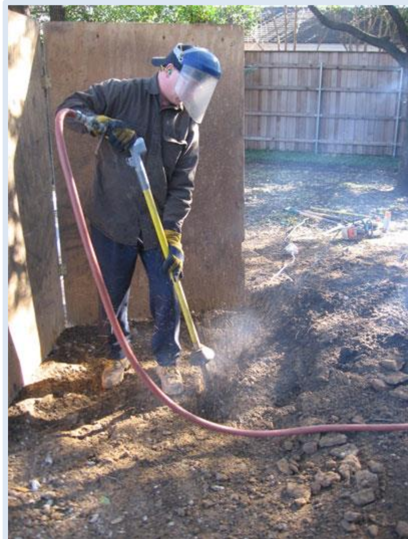
A high-pressure air tool can be used to safely remove excess soil from roots or a trunk
